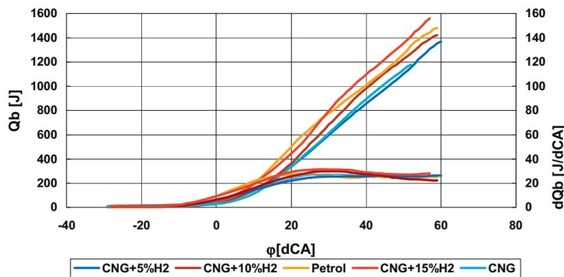
Fig. 8. Heat release and heat release rate as a function of crank angle for rpm = 2500 and full load
