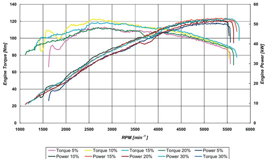
Fig. 4. Engine power and torque for all fuels
