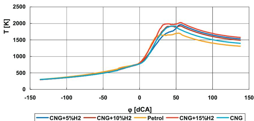
Fig. 6. Mean burned temperature as a function of crank angle for rpm = 2500 and full load
