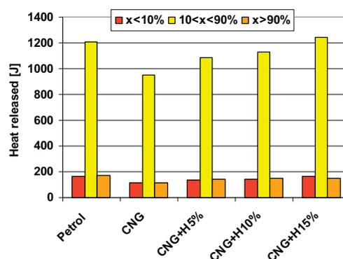
Fig. 11. Energy amounts produced in subsequent combustion process phases
