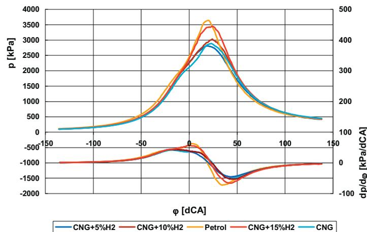
Fig. 5. Cylinder pressure and rate of pressure rise as a function of crank angle for tested engine ( for rpm = 2500 and full load)
