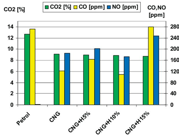
Fig. 9. Calculated CO<sub>2</sub>, NO and CO emission
