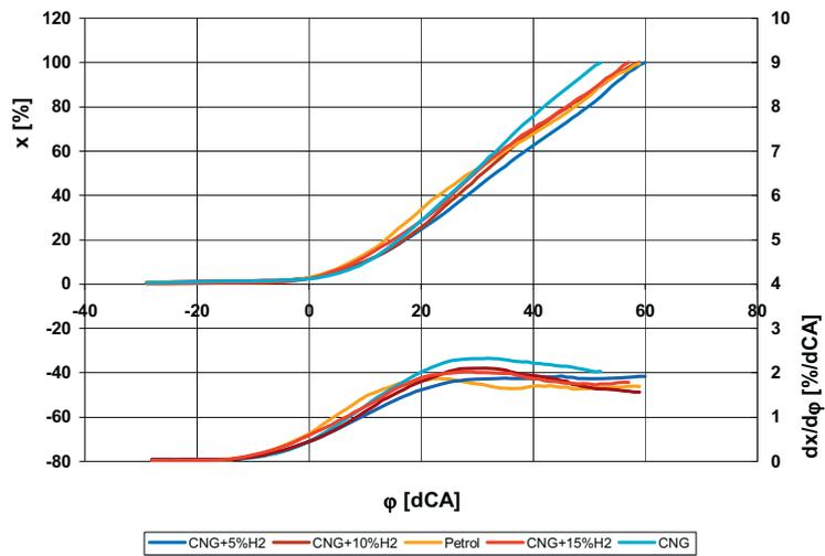
Fig. 7. Mass fraction burned and ratio of mass fraction burned rise as a function of CA for rpm = 2500 and full load
