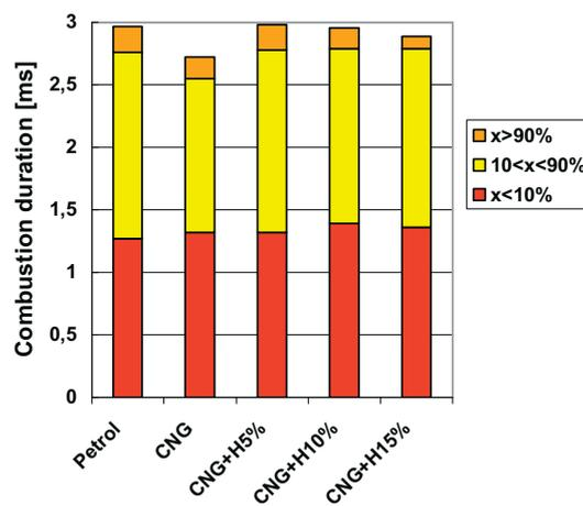
Fig. 10. Comparison of combustion duration of all fuels used during tests for rpm = 2500 and full load
